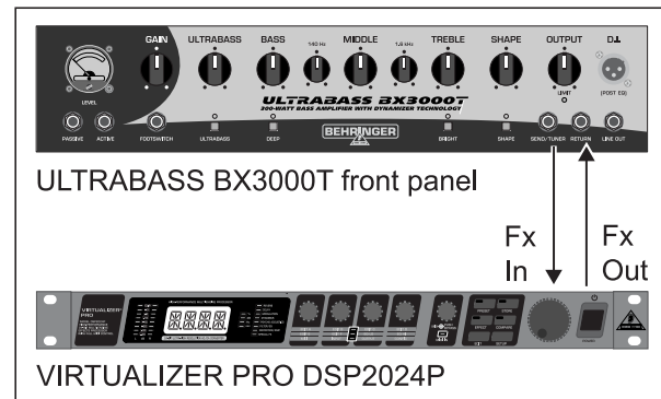
Fig. 3.4: Connection of a multi-effects processor
